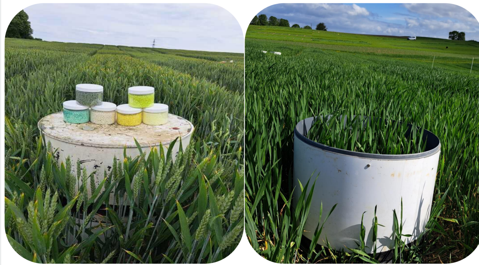
Figure 2: Measurement method (left: static N 2 O-N chamber and different applied N fertilizers, right: spacer for the N 2 O-N measuring system).
